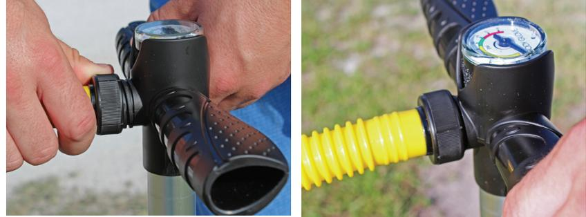
**STEP 5 :** Switch the pump from Single Action (1) to Dual Action (2) for quicker inflation of the board. The switch is located at the top of the pump cylinder. In this position the pump pushes air through the hose during both the downward push and upward pull.
